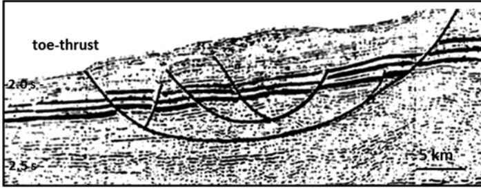
Fig. 4.8 A seismic segment showing an expression of a cylindrical fault which often occurs at slope margin. The fault is caused by excessive loading of finer clastics resulting in slope failure and attendant gravitational sliding of the sediments along the fault plane. The fault is often typified by small thrusts at the distal end (toe thrust) caused by resistance offered by the mobile shale mass (Image: courtesy ONGC, India)
