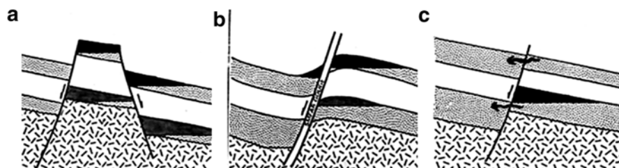
Fig. 5.2 Sketches illustrating fault properties. (a) Faults act as seal when the impermeable rock is juxtaposed to the reservoir, (b) faults occurring post entrapment may cause separate contacts in the faulted blocks when the fault plane gouge acts as lateral seal and (c) faults may cause hydrocarbons to leak partly or completely depending on occurrence of partial or no trapping due to permeable rocks set against reservoir (Modified after Harding and Tuminas 1989)
